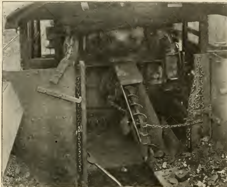
CROSBY STOKER, VIEW OF THE WORM CONVEYOR.
